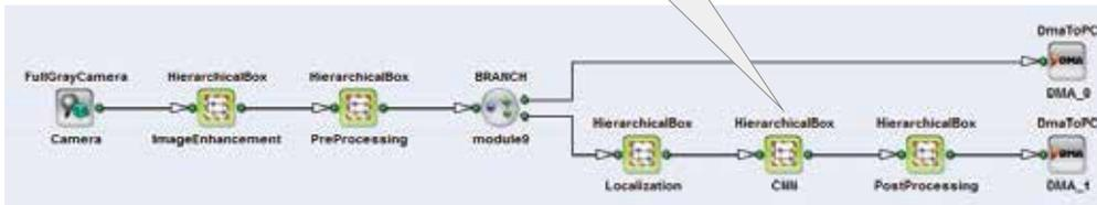
**CNN operator in Visual-Applets for various neural networks' architectures and weight/Source: Silicon Software GmbH**
