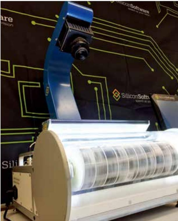
**Deep Learning application (error detection on metallic surfaces) running on a FPGA with a high data rate of approx. 200 MByte/s. / Source: Silicon Software GmbH**
