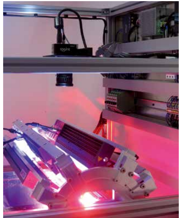
Arrangement of line lighting along the linear axis/ Source: MSTVision GmbH
