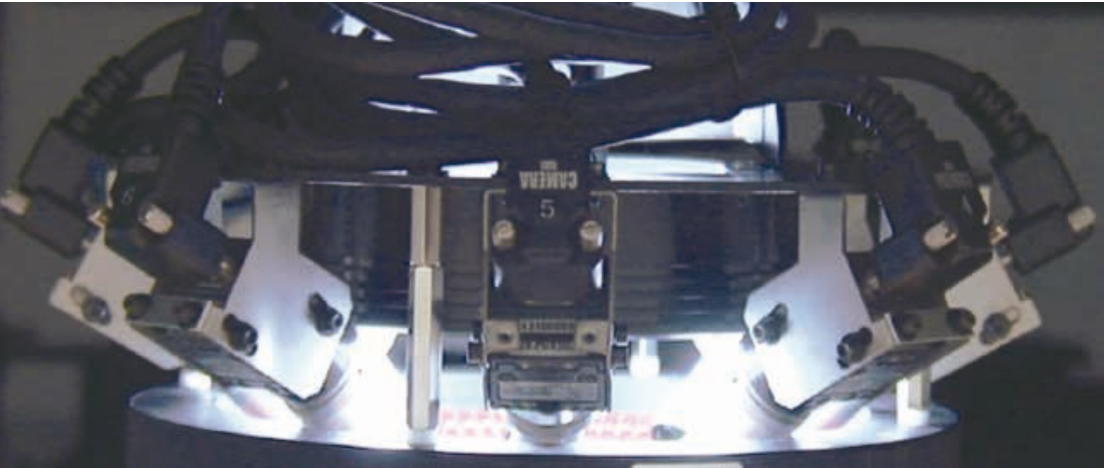
Optical unit in the inspection device with nine cameras/ Photo: MEK Marantz Electronics
