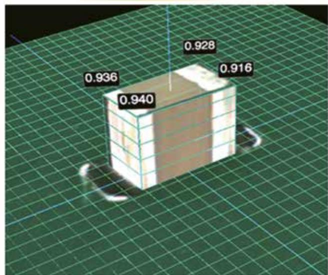
3D inspection of components and solder joints/ Photo: MEK Marantz Electronics
