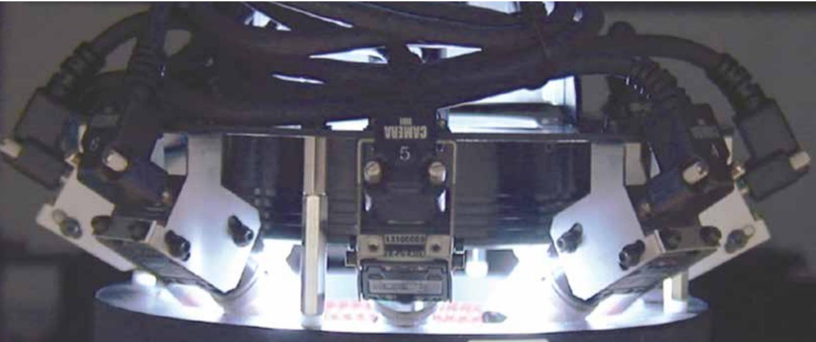
*Optical unit in the inspection device with nine cameras/ Source: MEK Marantz Electronics*
