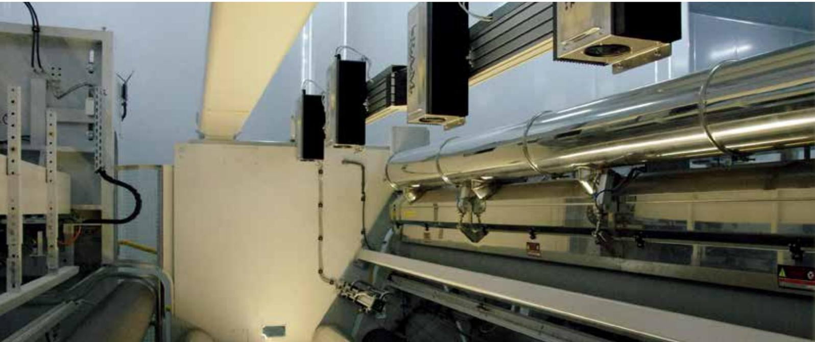
**Foil inspection system with 4x 8K cameras for the analysis of a 5.50 m large foil / Photo: R.A.M.**
